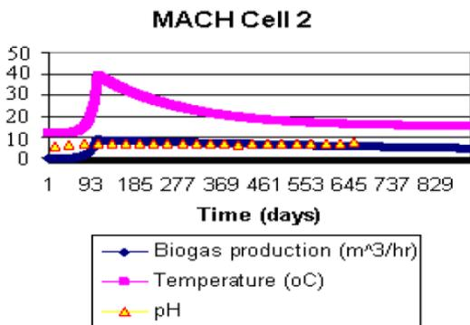
**Figure 4.** Biogas production and biodegradation characteristics at MACH's cell 2. Source: [31]
