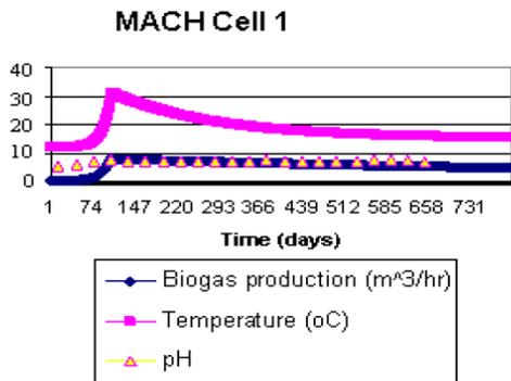
**Figure 3.** Biogas production and biodegradation characteristics at MACH's cell 1. Source: [31]
