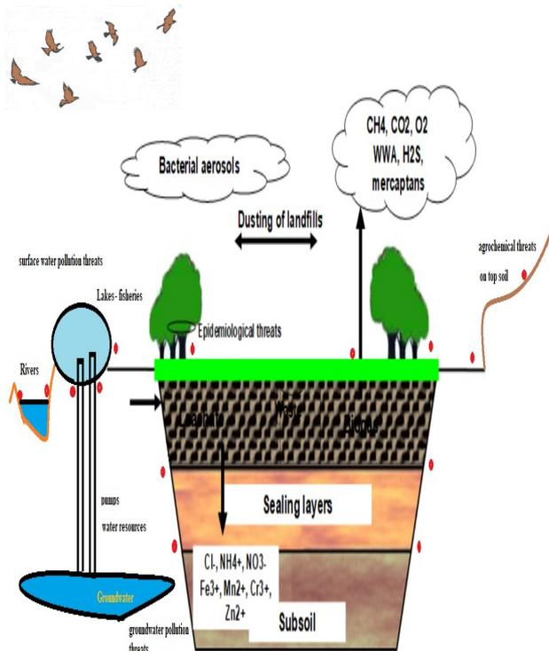
**Figure 2.** Sanitary drawing for monitoring locations next to landfills for environmental impact assessment of landfill emissions (red color bullets determine monitoring locations).
