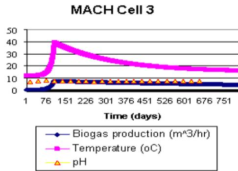
**Figure 5.** Biogas production and biodegradation characteristics at MACH's cell 3. Source: [31]
