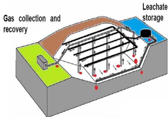
**Figure 6.** Sanitary drawing for monitoring schemes at landfills protecting flora and fauna resources next to landfill boundaries, (red color bullets determine the monitoring points).
