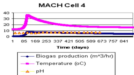
**Figure 6.** Biogas production and biodegradation characteristics at MACH's cell 4. Source: [31]
